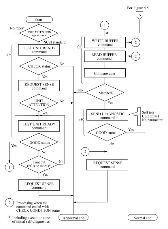
Figure 5.4 Checking the SCSI connection (A)
